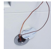
Cable port in the side wall
