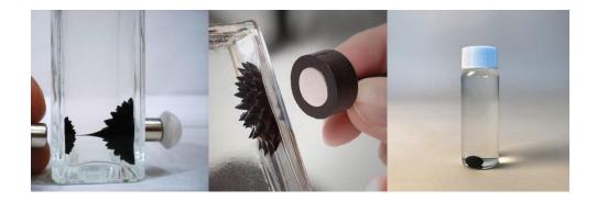
The product provides movement and understanding the principle of magnetic fluid by inserting fills and magnetic fluids. Using magnets to observe spikes in magnetic fluid by moving magnet.
