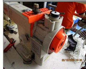
Photo of the personal protection equipments (if applicable) Pulley guard for sewing machine.JPG
